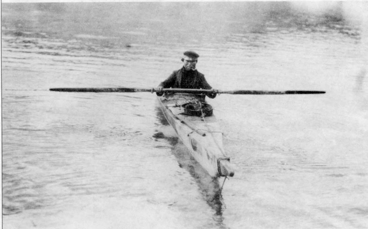
Eskimo paddler from Lake Harbour, Baffin Island. Note typical long-bladed East Arctic paddle with drip rings. Courtesy Public Archives of Canada.
