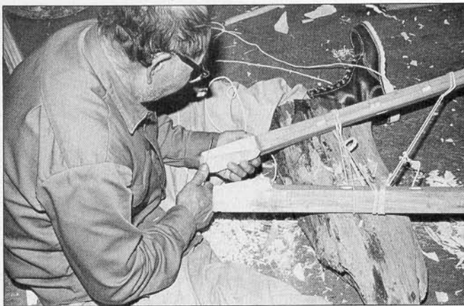
Left—The gunwales were fashioned from a driftwood log, squared up with a hatchet and adze, halved with a circular saw, and carved to fit.
