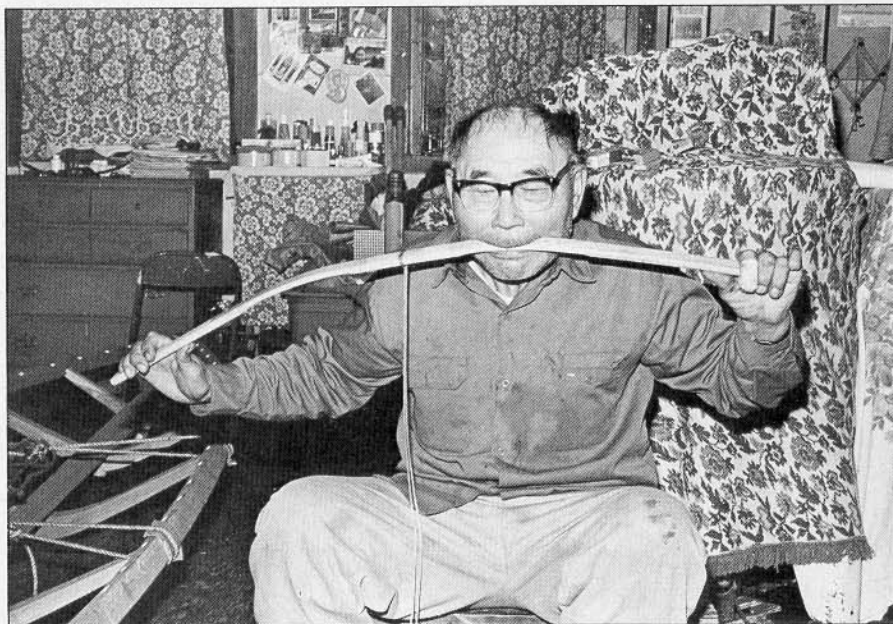
Below—Dick Bunyan bending a kayak rib without steaming it. His teeth act as a clamp to prevent the outer fibers from splitting while crushing the inboard ones to facilitate bending.
