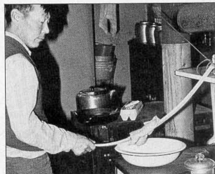
Above—Aloysius Hale puts hot water on the outer cockpit coaming rim to bend it.
