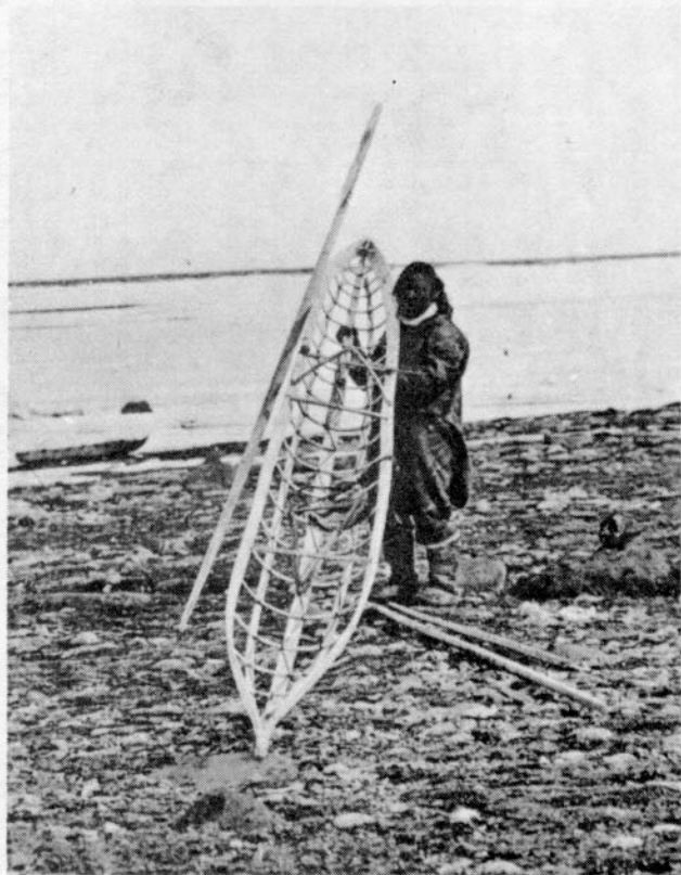
PHOTO 2: CRUDELY CONSTRUCTED KAYAK FRAME FROM BERNARD HARBOUR, CORONATION GULF. NOTE THAT SEVERAL DECK BEAMS, THE DECK STRINGER AND THE COCKPIT COAMING ARE MISSING. Photo 36977, Courtesy National Museums of Canada.
