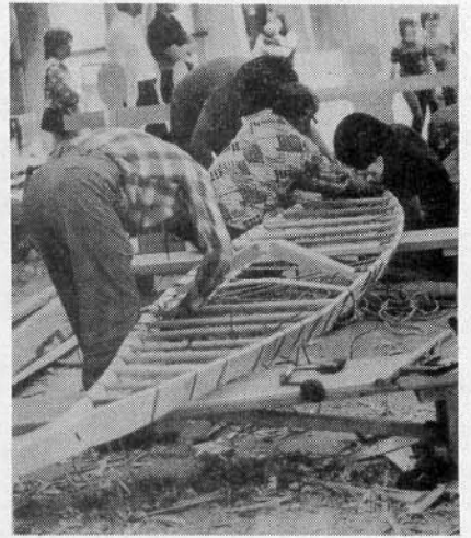
Figure 3 THE HEAVY GUNWALES ARE THE MAIN STRENGTH MEMBERS AND ARE HELD APART BY 17 DECK BEAMS MORTISED INTO THE GUNWALES. THE CURVED DECKBEAM JUST FORWARD OF THE COCKPIT COAMING IS CARVED FROM A SINGLE PIECE OF WOOD FOR MAXIMUM STRENGTH.
