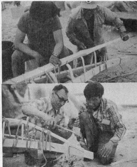
Figures 7 & 8 THE NEXT STEP IN CONSTRUCTION INVOLVES CARVING LONG, SLIGHTLY HOLLOWED LONGITUDINAL STRINGERS THAT ARE FITTED AND LASHED TO THE RIBS AT THE CHINE OR TURN-OF-THE-BILGE. IN THE AREA WHERE THE KAYAKER SITS, ADDITIONAL LONGITUDINAL STRINGERS ARE LASHED BETWEEN THE KEELSON AND BILGE STRINGERS.
