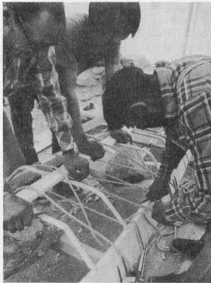
Figures 4, 5, & 6 THE COMPLETED LADDER-LIKE FRAME IS TURNED UPSIDE DOWN. SEVERAL KEY RIBS ARE FITTED INTO MORTISES IN THE GUNWALES. THE KEELSON IS TEMPORARILY LASHED ON TO GIVE THE BOTTOM ITS PROFILE FORM. THE REMAINING RIBS ARE FITTED UNDER THE KEELSON, AFTER WHICH THE ENDS OF THE KEELSON ARE PERMANENTLY LASHED TO THE GUNWALES.
